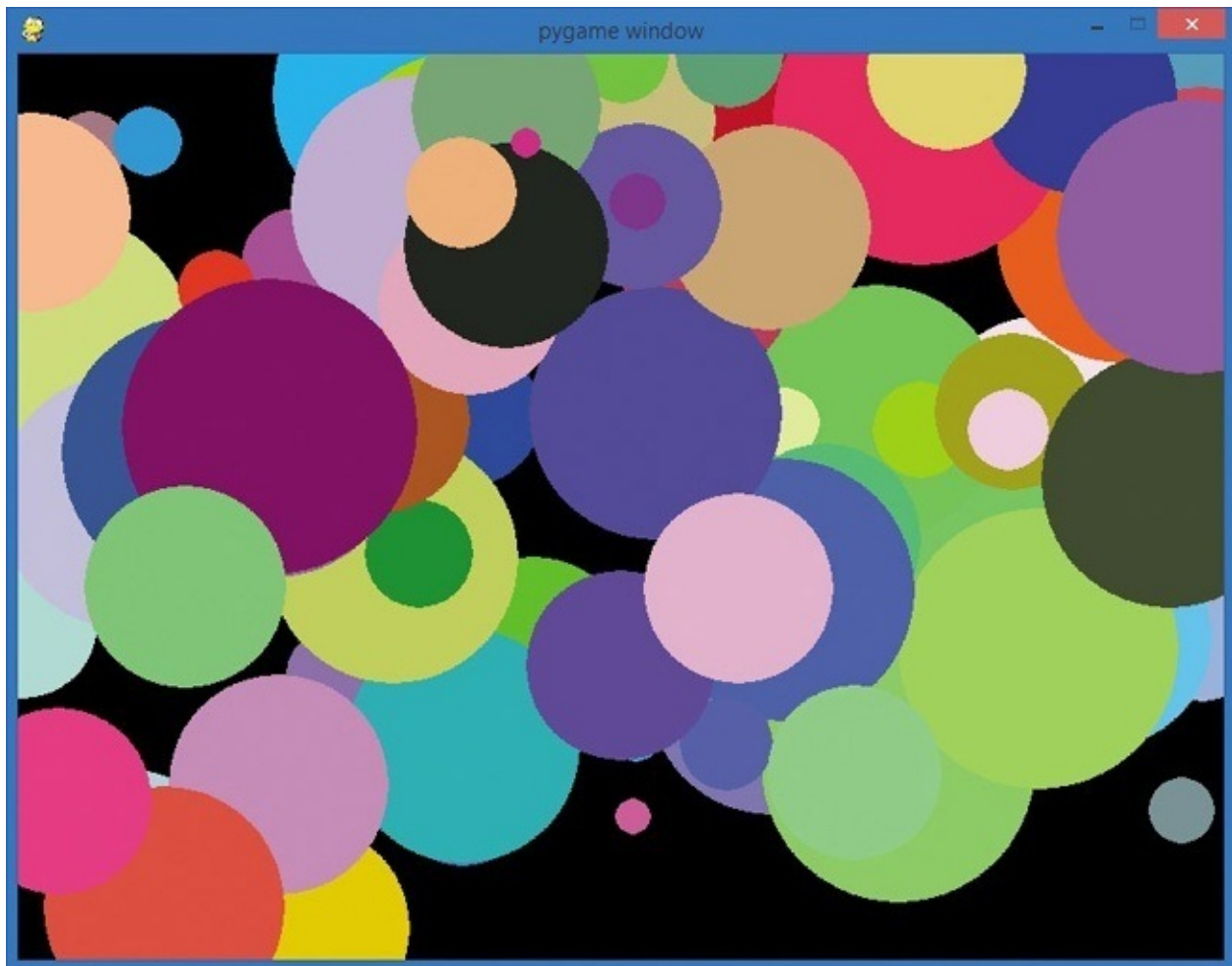
Figure 8-10. An advanced version of our dot program, RandomDots.py , gives us 100 dots of random color, location, and size.
