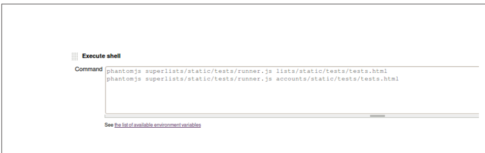
Figure 20-12. Add a build step for our JavaScript unit tests
