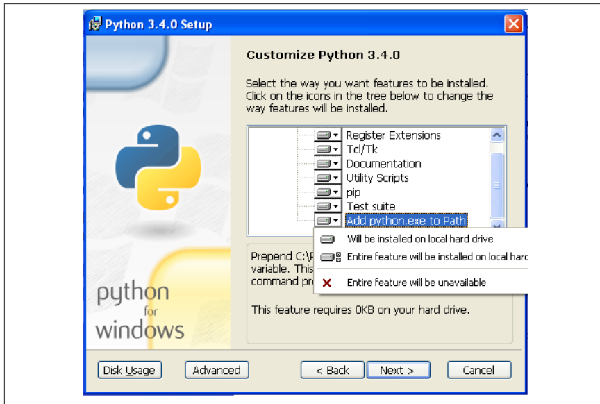
Figure P-1. Add python to the system path from the installer
